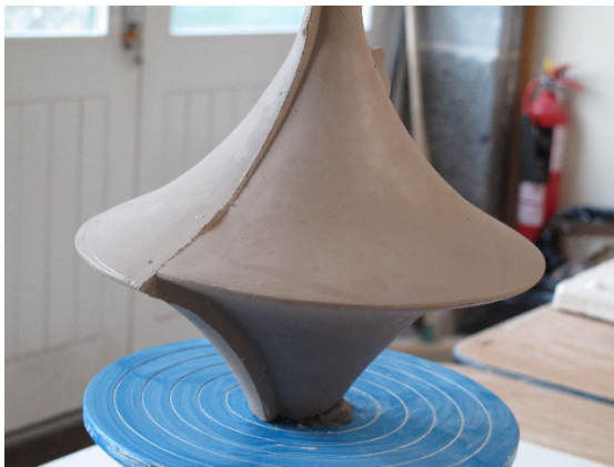
Fig. 30.2 Kathleen Moroney (2010). Misaligned form created during the pouring of clay into a misaligned plaster mould, resulting in large disconnected seams on the side of the form.
