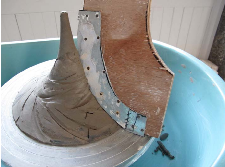
Fig. 29.1 Kathleen Moroney (2010). Metal template pushed against clay form creating textural effect in the clay as the wheel turns.
